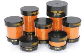
D-Series Breathers feature numerous models in a variety of sizes, all designed to satisfy the requirements of most stationary fluid management applications. The breathers provide application flexibility by using 100% silica gel for moisture adsorption, 100% activated carbon for fume and odor control or both, when necessary. All D-Series models feature 2-micron solid particle filtration and are available with airflow ratings of 20 cfm.
