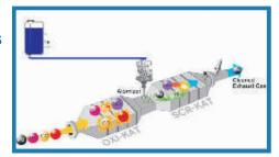
SCR systems are extremely sensitive to potential chemical impurities in the urea solution. In order to ensure that the SCR system continues to work effectively, care must be taken to ensure the purity of the catalyst and the reducing agent. Even small amounts of contaminant can severely impact the performance of the SCR system.
