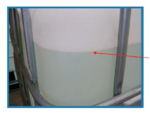
If there is a film or scum on the surface of the liquid then don't use it. Likewise if the liquid looks cloudy and discoloured. These are signs of contamination and increasing the risk of damaging the SCR System.
