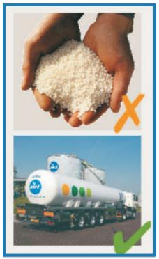
There are basically two methods used to manufacture AdBlue. The 'Hot-Melt' Virgin Urea production method is widely accepted across the industry as producing the highest purity grade of AdBlue. This is because it eliminates the risk of contamination during manufacture. The urea is in its 'virgin' liquid state when it is combined with the deionised water so there is no chance of contaminants being introduced during manufacture.
