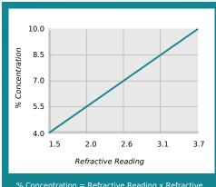
% Concentration = Refractive Reading x Refractive Factor Coolant Refractometer Factor % Brix = 2.7
