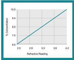
% Concentration = Refractive Reading x Refractive Factor Coolant Refractometer Factor % Brix = 2.4
