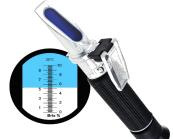
A traditional handheld refractometer is an analog instrument for measuring a liquid's refractive index. It works on the critical angle principle by which lenses and prisms project a shadow line onto a small glass reticle inside the instrument, which is then viewed by the user through a magnifying eyepiece.
